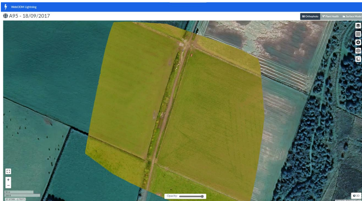
Figure 17. Orthomosaic photo created with WebODM using 183 Knock Farm drone images.
